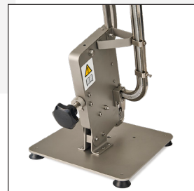
Control of the clip closure with the eccentric mechanism.
